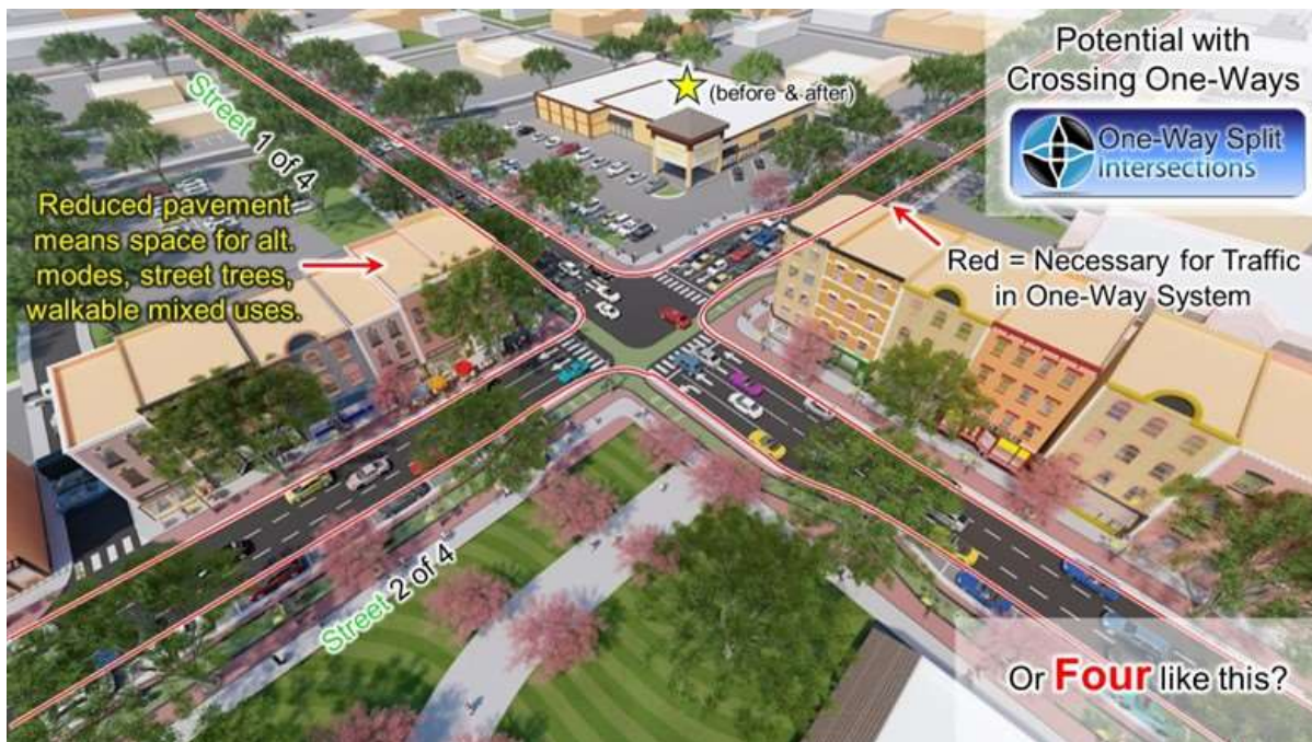
Figure 5-12 Same Location, Reconfigured with four One-Way Streets
