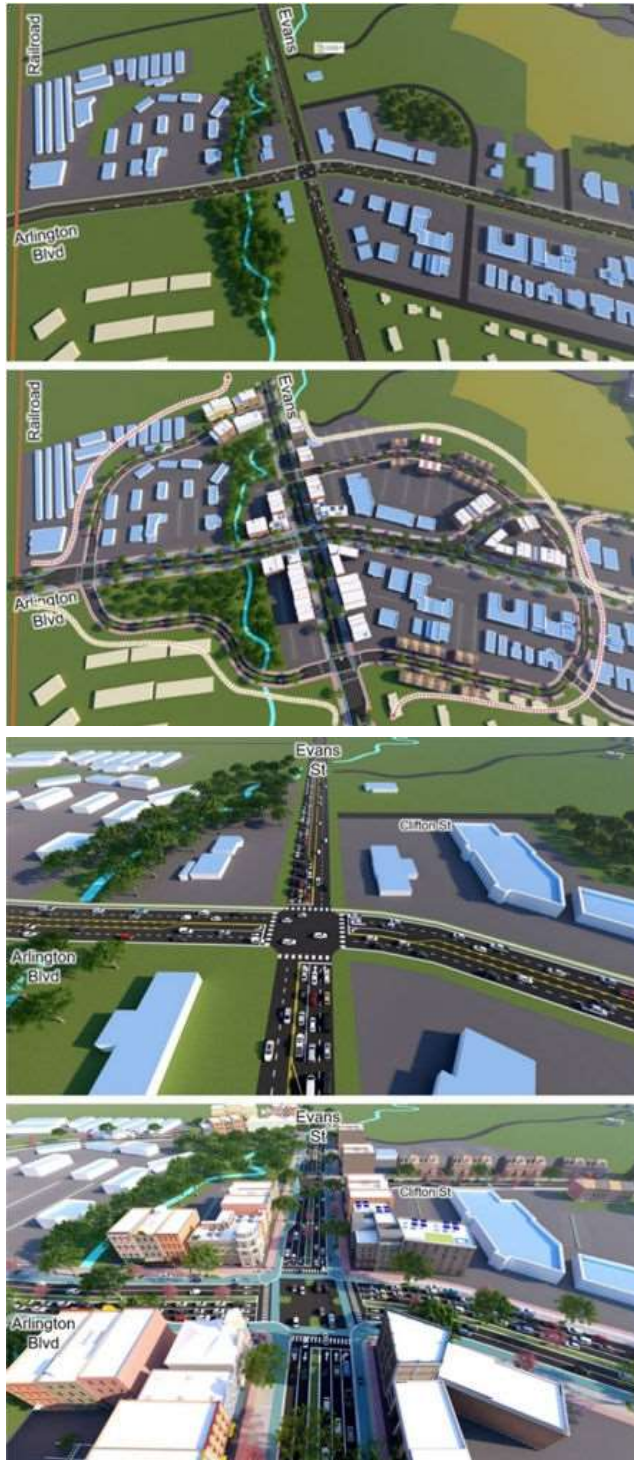
Figure 8-13 Before / After Quadrant Intersection
