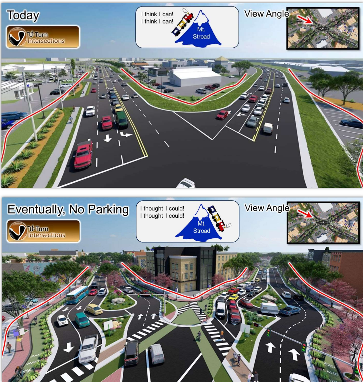
Figure 4-10 Birdseye view of U-Turn design. Chicanes near intersection ensure safer speeds at crossing.
